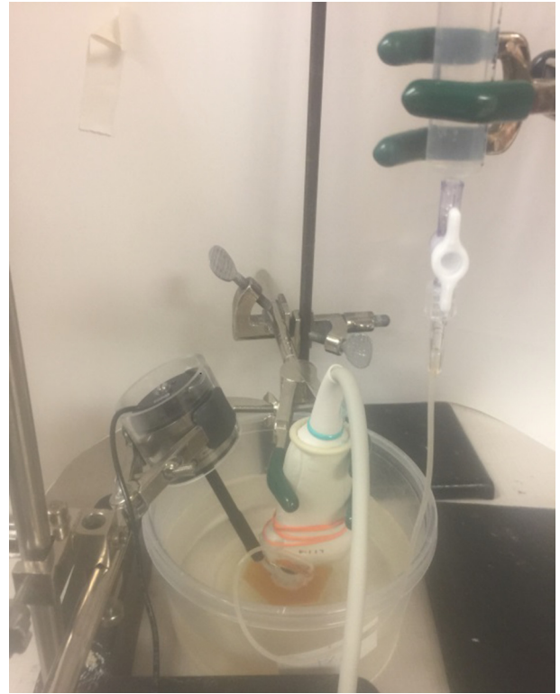
Fig. 1. Experimental setup of the USWE system. The shaker was in touch with the limbus region of eye ball to generate a 0.1 s harmonic vibration while an ultrasound probe was placed over the eye ball to measure the wave speed of cornea noninvasively. A butterfly needle was inserted in the vitreous region of the eyeball with the ultrasound imaging guidance. The needle was connected to a syringe filled with water. The IOP was obtained by the water column height of the syringe relative to the water level in the testing container. The IOP was changed from 5 mmHg to 30 mmHg with an interval of 5 mmHg.
